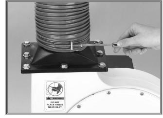
Figure 17. Securing transfer hose with clamp.
